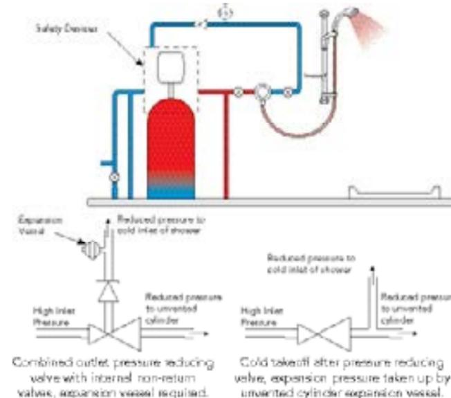
An Unvented cylinder provides a known volume of stored hot water usually at temperatures between 55 to 65°C. Water can be heated by electric immersion heater, central heating indirect coil or gas and oil burner direct flame.
